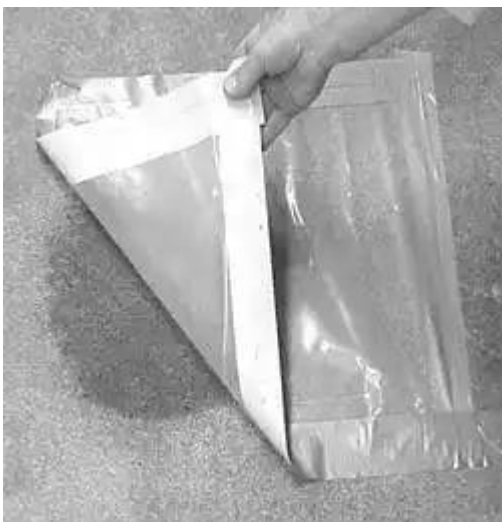
Pic 4 Checking the substrate to see if moisture present, which in this case is. You can see the dark moist surface. Also, there is likely moisture droplets on underside of the plastic sheet. Allow substrate to dry completely if in doubt.
